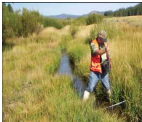
Seepage Run Streamflow Measurement, September 2011
