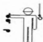
**Raise the Boom and Lower the Load:** Arm extended, fingers closed, thumb pointing
