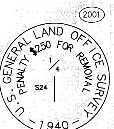
2001 FOUND 2 1/4" IRON PIPE WITH 2 1/2" BRASS CAP, STAMPED AS SHOWN IN SMALL ROCK MOUND PER 7 RS 94. THE PIPE IS BENT OVER TO THE SOUTH. DUG DOWN AND LOCATED BASE OF PIPE, WHICH IS STILL SOLID. ACCEPTED AS EAST 1/4 CORNER OF SECTION 24, TOWNSHIP 26 NORTH, RANGE 8 EAST, MOUNT DIABLO MERIDIAN.
