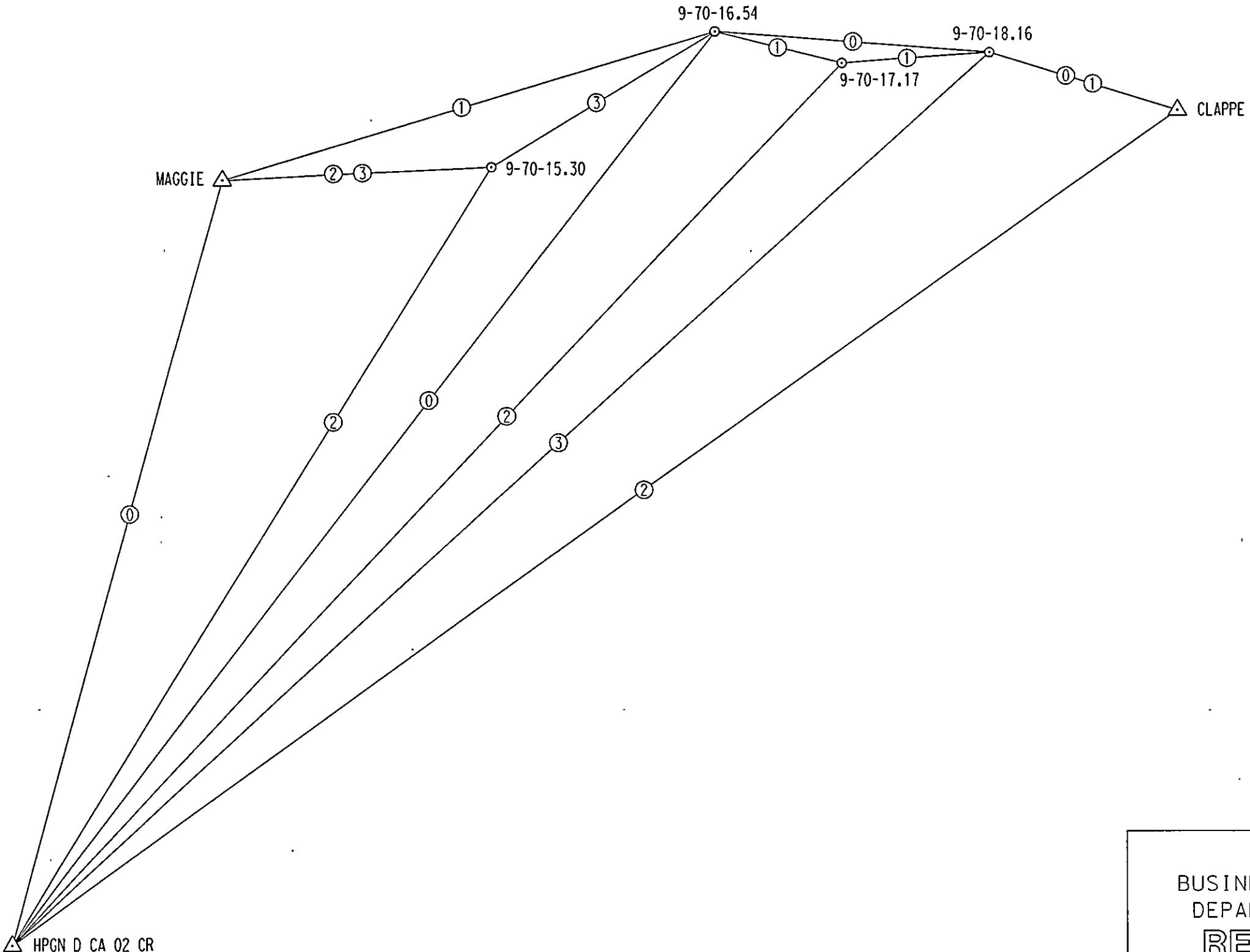
BEARINGS, DISTANCES, AND COORDINATES ARE BASED ON THE CALIFORNIA COORDINATE SYSTEM OF 1983, ZONE 1, EPOCH 2004.69-CCS 83 ZONE 1 (2004.69)
