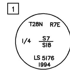
Found Axle and a 1" dia. Iron Pipe L.S. 3202 along side, 4" under asphalt. Set a 2 1/2" dia. aluminum cap over the above in cement flush to pavement.
