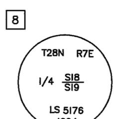
Found a 1 1/4" dia. Iron Pipe L.S. 2322. Set a Standard U.S.D.A. Monument 24" in ground 4" above in a 1 1/2" dia. stone mound. Emplaced above monument inside.
