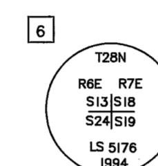
Found a 1" dia. Iron Pipe R.C.E. 7567, 8" above ground in a 1' dia stone mound. Set a Standard U.S.D.A. Monument 23" in ground 5" above in a 1 1/2" dia. stone mound. Emplaced the above monument inside.
