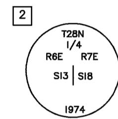
Found B.L.M. Brass Cap 4" above ground in a 1 1/2" dia. stone mound. A 1" dia. Iron Pipe R.C.E. 7567 along side.
