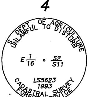
5 RECORD: POST 4 FT LONG, 4 IN DIA 2 FT DEEP IN A STONE MOUND, 4 1/2 FT IN DIA AT BASE, 2 FT HIGH, FOR CORNER TO SECTIONS 1, 2, 11, AND 12.
