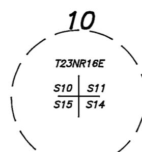
10 RECORD: POST 4 FT LONG AND 4" DIA., FOR CORNER TO SECTIONS 10, 11, 14, AND 15
