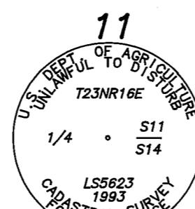
11 RECORD: SET POST FOR CORNER TO FRACTIONAL SECTIONS 11 AND 14, WITH MOUND, PITS AND TRENCH, AS PER INSTRUCTIONS
