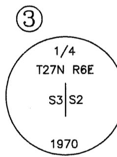
Found a BLM Brass Cap in a 2 1/2' dia. by 6" high stone mound. Cap Marked:
