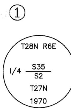
Found a BLM Brass Cap in a 6" high by 3' dia. stone mound, with a 2" iron pipe, LS Tag 2322 along side. Cap marked:
