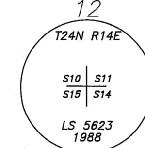
RECORD: (GLO) SET VOLCANIC STONE 20X15X10 IN STONE MOUND 5 FEET IN DIAMETER AT BASE AND 2 FEET HIGH FOR CORNER TO SECTIONS 10,11,14,15.
