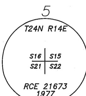
RECORD: (GLO) SET A POST 5 FEET LONG, 4 INCHES DIAMETER AND 2 FEET DEEP IN A MOUND 4 1/2 FEET IN DIAMETER AT BASE AND 2 FEET HIGH FOR CORNER TO SECTIONS 15,16,21,22 WITH PITS 24X18X12.
