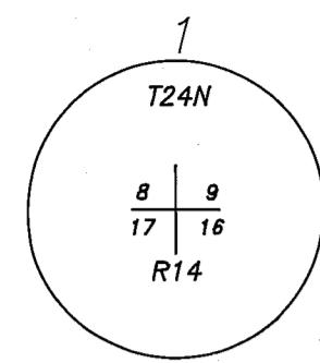
RECORD: (GLO) SET A POST 5 FEET LONG AND 4 INCHES DIAMETER, 2 FEET DEEP IN A MOUND 4 1/2 FEET IN DIAMETER AT BASE AND 2 FEET HIGH WITH PITS 24X18X12 FOR CORNER TO SECTIONS 8,9,16,17.
