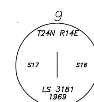
RECORD: (GLO) SET A POST 4 FEET LONG AND 4 INCHES IN DIAMETER, 2 FEET DEEP IN A MOUND 4 1/2 FEET IN DIAMETER AT BASE AND 2 FEET HIGH WITH PITS 24X18X12 FOR QUARTER SECTION CORNER.
