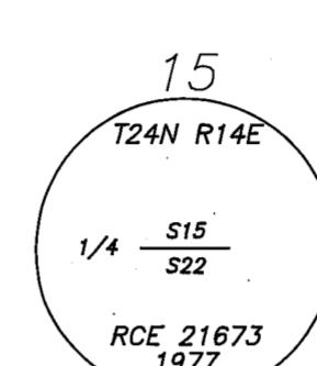
RECORD: (GLO) SET A POST 4 FEET LONG 4 INCHES DIAMETER 2 FEET DEEP IN A MOUND 4 1/2 FEET IN DIAMETER AT BASE AND 2 FEET HIGH WITH PITS 24X18X12 FOR QUARTER SECTION CORNER.
