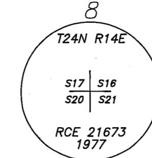
RECORD: (GLO) SET A STONE 24X15X6 IN A STONE MOUND 4 1/2 FEET IN DIAMETER AT BASE AND 2 FEET HIGH FOR CORNER TO SECTIONS 16,17,20,21 ON A BED OF ROCKS.
