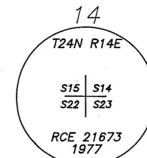
RECORD: (GLO) SET A POST 5 FEET LONG AND 4 INCHES DIAMETER AND 2 FEET DEEP FOR CORNER TO SECTIONS 14,15,22,23 FROM WHICH FWB:
