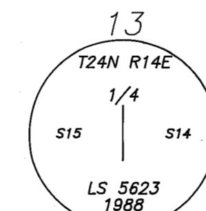
RECORD: (GLO) SET A STONE 15X12X6 IN A STONE MOUND 4 1/2 FEET IN DIAMETER AT BASE AND 2 FEET HIGH FOR QUARTER SECTION CORNER ON A BED OF ROCKS.
