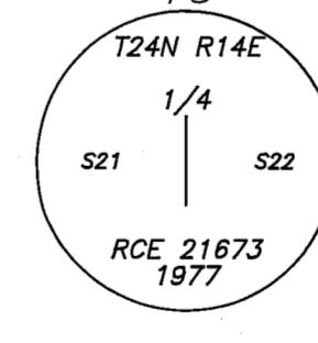
RECORD: (GLO) SET STONE 20X15X12 IN A STONE MOUND 4 1/2 FEET IN DIAMETER AT BASE AND 2 FEET HIGH FOR QUARTER SECTION CORNER.
