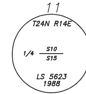
RECORD: (GLO) SET A POST 4 FEET LONG AND 4 INCHES DIAMETER 2 FEET DEEP IN A MOUND 4 1/2 FEET IN DIAMETER AT BASE AND 2 FEET HIGH WITH PITS 24X18X12 FOR QUARTER SECTION CORNER.
