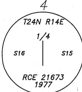
RECORD: (GLO) SET A POST 4 FEET LONG AND 4 INCHES DIAMETER 2 FEET DEEP IN A MOUND 4 1/2 FEET DIAMETER AT BASE AND 2 FEET HIGH WITH PITS 24X18X12 FOR QUARTER SECTION CORNER.
