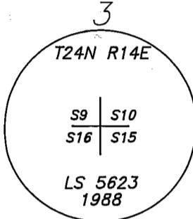
RECORD: (GLO) SET A POST 5 FEET LONG AND 5 INCHES DIAMETER, 2 FEET IN A MOUND 4 1/2 FEET IN DIAMETER AT BASE AND 2 FEET HIGH WITH PITS 24X18X12 FOR CORNER TO SECTIONS 9,10,15,16.
