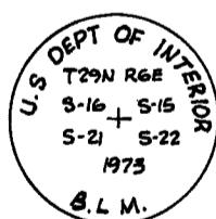
Fd. 2 1/2" Iron Pipe and Brass Cap set flush in sand bar 12 1/2' east of easterly edge of Warner Creek per B.L.M. corner remonumentation notes dated June, 1973, marked as shown for corner common to Sections 15, 16, 21 and 22, T 29 N, R 6 E, M.D.M., with all bearing trees referred to in said notes existing. B.L.M. File No. CSO-9180-15, June, 1973.
