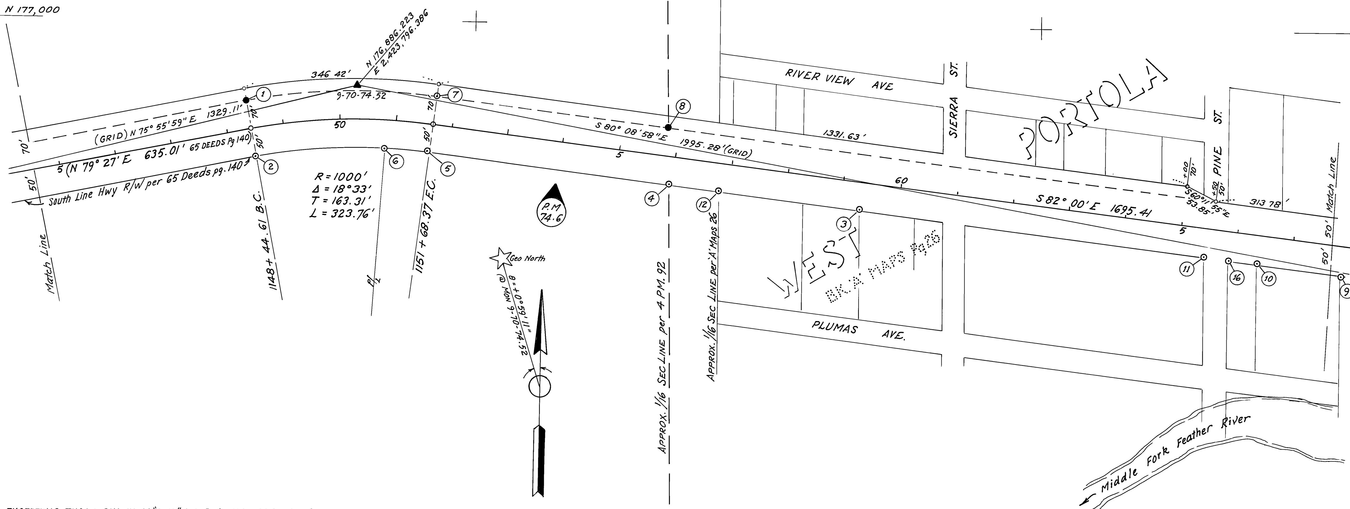
EXCEPTING THOSE SHOWN AS "GRID" ALL BEARINGS ARE BASED ON THE CENTERLINE OF STATE HIGHWAY PER BK 65 DEEDS Pg 140 AND Pg. 427.
