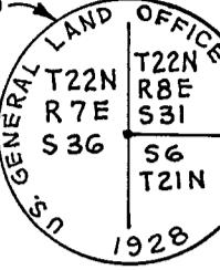
10. SET TOPPER IN 2 FOOT HIGH STONE MOUND, MARKED 1/4 SEC. COR. FOR CORNER COMMON TO SEC. 31, T.22N., R.8E., M.D.M. AND SEC. 6, T.21N., R.8E., M.D.M. NO EVIDENCE EXISTING OF ORIGINAL CORNER; FROM WHICH AN 18" FIR BEARING TREE BEARS N 31° 09' W 30.0 FEET DISTANT, AND AN 18" FIR BEARING TREE BEARS S 03° 37' E 38.3 FEET DISTANT.
