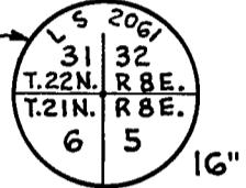
12. SET TOPPER IN 2 FOOT HIGH STONE MOUND, MARKED 1/4 SEC. COR. COMMON TO SEC. 32, T.22N., R.8E. AND T.21N., R.8E., NO EVIDENCE EXISTING OF ORIGINAL CORNER, FROM WHICH A 20" FIR BEARING TREE BEARS N. 11° 44' W. 50.5 FEET DISTANT AND A 14" FIR BEARING TREE BEARS S 33° 14' E 36.9 FEET DISTANT.
