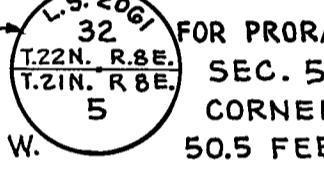
13. FOUND POST AND STONE MOUND ON STUMP. FOREST SERVICE PLATES ON ADJACENT TREES IDENTIFY THIS AS BEING THE CORNER OF T.22N., R.8E., M.D.M. SET TOPPER AND STONE MOUND AT POST MARKED FROM WHICH AN OLD BEARING TREE, 60" DIA. PINE, BEARS N 44° 18' W 37.0 FEET DISTANT, AND A BEARING TREE, 20" DIA. FIR, BEARS S 41° 08' W 17.5 FEET DISTANT, AND A BEARING TREE, 16" DIA. FIR, BEARS N 36° 24' E 5.5 FEET DISTANT.
