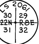
3. FOUND 21" x 24" GRANITE STONE, RED PAINTED. FOREST SERVICE PLATES ON TWO (2) ADJACENT TREES, EACH MARKED FOR "32 | 29 T.22N., R.8E." SET TOPPER IN 2' HIGH STONE MOUND MARKED FROM WHICH A BEARING TREE, 13" DIA. FIR, BEARS S 11° 45' E 5.1 FEET DISTANT, AND A BEARING TREE, 12" DIA. FIR, BEARS N 08° 15' W 11.8 FEET DISTANT.
