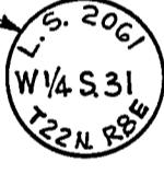
8. FOUND 2" DIA. IRON PIPE IN RED PAINTED STONE MOUND WITH 2 1/2" CAP, FOREST SERVICE PLATE ON ADJACENT TREE, FOR ANGLE POINT ON WEST LINE SEC. 31, T.22N., R.8E., M.D.M.
