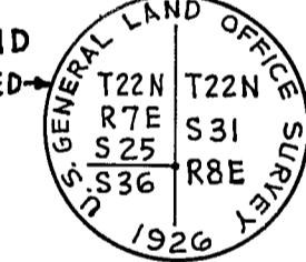
4. FOUND 4" DIA. TOP x 14" DIA. BASE x 16" HIGH LAVA STONE IN STONE MOUND. FOREST SERVICE PLATES ON TWO (2) ADJACENT TREES, EACH MARKED FOR "32 | 29 T.22N., R.8E." SET TOPPER MARKED "29 | 28" IN 2' HIGH STONE MOUND FROM WHICH A BEARING TREE, 25" DIA. FIR, BEARS N 02° 45' E 13.7 FEET DISTANT, AND A BEARING TREE, 22" DIA. FIR, BEARS N 43° 45' E 17.0 FEET DISTANT.
